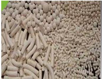
**PSA plant** employs **Zeolite** molecular sieves to separate the **oxygen** from the air. **Oxygen** with high purity is delivered whereas the nitrogen adsorbed by the molecular sieves is sent back into the air through the exhaust pipe. Pressure swing adsorption (**PSA**) process comprises of two vessels filled with molecular sieves and activated alumina.
